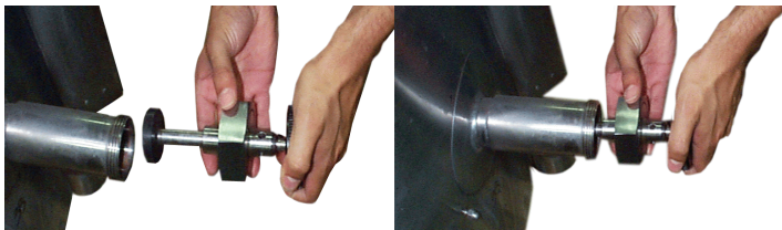
Assemble and attach the tangent draw-off valve after the kettle is unpacked.
