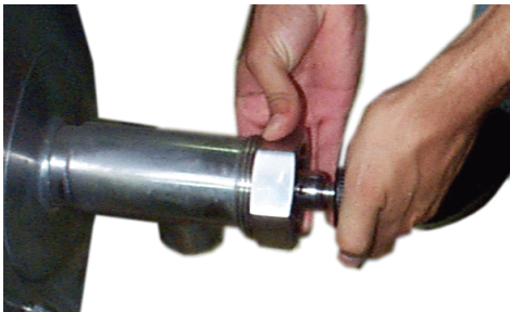
When attaching the draw-off valve, just hand-tighten the nut.
