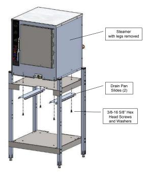
2.3 [NOTE: the following step is optional – the machine screws are not needed for structural integrity of the steamer or the stand.]
