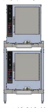
2.6. Note that the steamers mount directly to the shelves and the drain pans (standard 12 x 20 x 4" hotel pan) slide into the rails mounted underneath the shelves.
