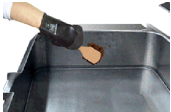
Use a brush, sponge, cloth, plastic or rubber scraper, or plastic wool to clean.
