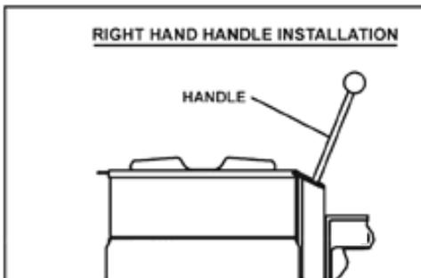
**NOTE:** After handle installation on the right hand side, retain the hardware supplied with the unit for left hand installation.
