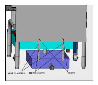
d. Fit the splash guard onto the drain cart hinge pins.
