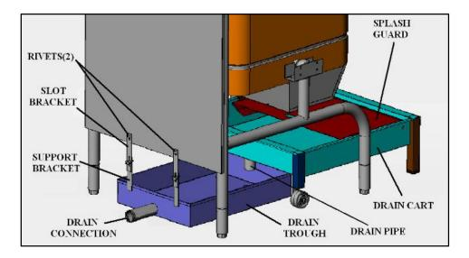
c. Slide the slot brackets over the rivets and adjust the height using the thumbscrews. Make sure to tighten thumbscrews down once the height has been set.
