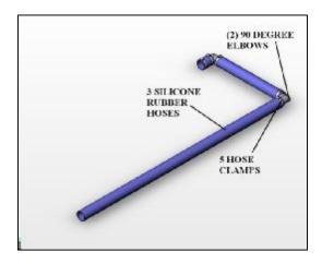
Once assembled as shown above, tighten the hose clamps around the edges of the 90 degree elbows. Position the opening of the 3-1/2" hose over the drain connection on the drain trough. Tighten and secure clamp around the hose and the drain connection as shown below.
