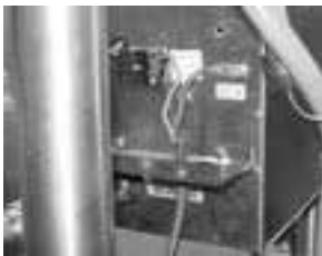
Electronic spark ignition
