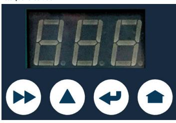
The PCD-2 makes use of only four buttons and a 3-digit LED display for all dispenser operation and programming.
