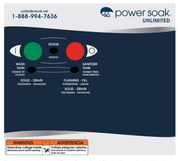
The illustration shows the PS-200 Control Panel Overlay. The overlay is adhered to the front of the control panel box and contains buttons and lights that are imbedded into the overlay. Communication with the UPM is accomplished with cables that extend from the back side of the overlay.
