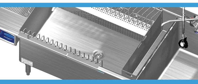
While the racking system holds the pans in place, Power Soak's patented, evenly spaced wash jets run along the back wall of the wash tank making it impossible to starve the Power Soak wash pump.
