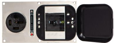
The **"point-of-use" breaker plate**, whether in the heavy-duty 5" x 9" version or the 4" x 12" modular version, is the heart of the Utility Distribution System. Since the circuit breaker and the matching outlet are on one plate, they travel together — whether to move, replace or add equipment. Each plate can be designed to accommodate any possible connection to serve the piece of equipment as needed.
