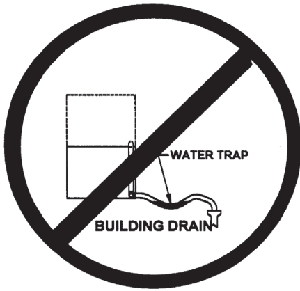
IMPROPER DRAIN LINE CONNECTION
