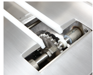
Sealed bearings require no lubrication
