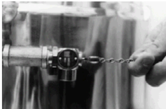
Test the safety valve each day
