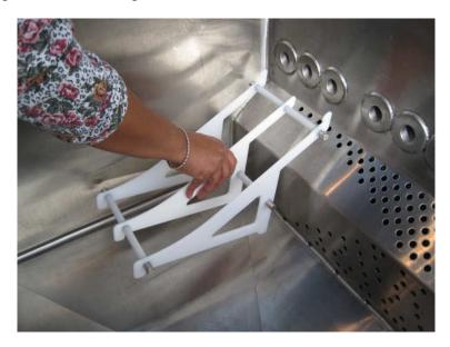
Place the other rear rib sets against the back wall of the sink leaving a finger-size gap between them.
