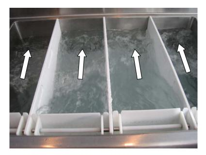
Do not place knives or other sharp objects in the Produce Soak. Allowing knives or other sharp objects to tumble freely in the Produce Soak tank may cause damage to the equipment and bodily injury to the user.
