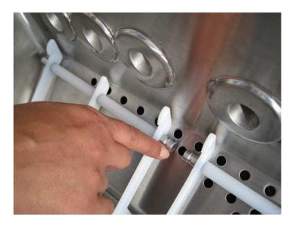
When you have placed all of the rear rib sets, begin placing front rib sets against the front wall of the sink. As with the rear rib sets, place the first front rib set against a corner, and leave a finger-size gap between it and the next front rib set.
