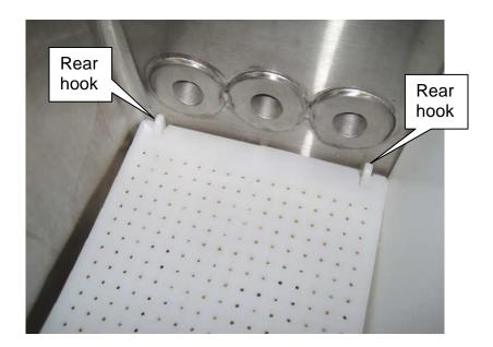
Continue to push the flow guide down against the rib sets until the notched end of the flow guide nearest you is adjacent to the hooks of the front rib set.
