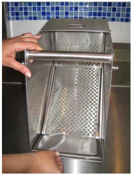
Allow a few minutes of collection time in each position. When finished, empty the contents of the filter into a suitable waste container, and wash out the filter and basket.
