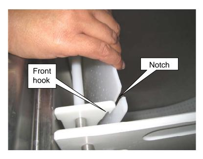
While holding the flow guide against the front rib set, rock the front rib set and the end of the flow guide away from you until the notches in the flow guide engage the hooks of the front rib set.
