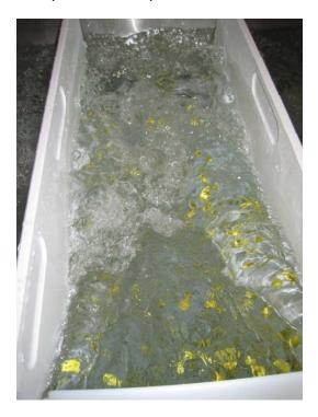
This can be done by placing a filter screen in a basket and then placing the basket in each of the four wash sections.
