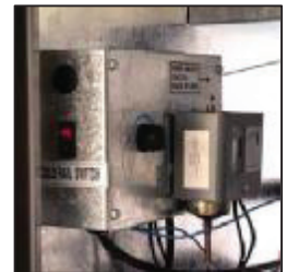
Rail thermostat and on/off switch are independent of base for energy savings
