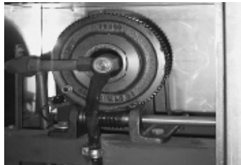
Liberal grease the wheel where it contacts the worm gear.
