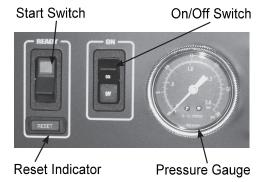
After the unit has been installed, test it to ensure that it is operating properly. Operating Controls are located on the front of the cabinet base unit.
