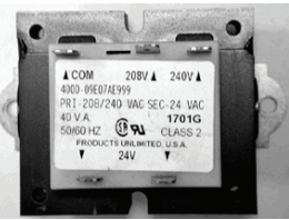
Pull lead from 208V tab and insert on 240V tab.
