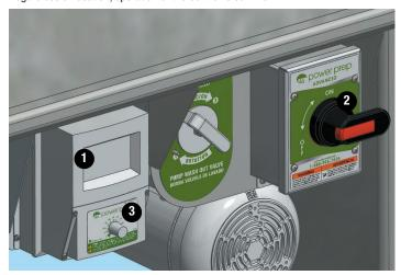
To start the flow, turn on the 2 power switch.
