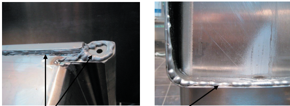
SEALANT APPLIED TO UNDERSIDE OF JBZ JOINT AND FACE OF THE END PLATE
